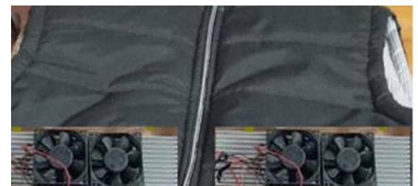
Figure 14 Prototype Concept of Peltier Module Integration
