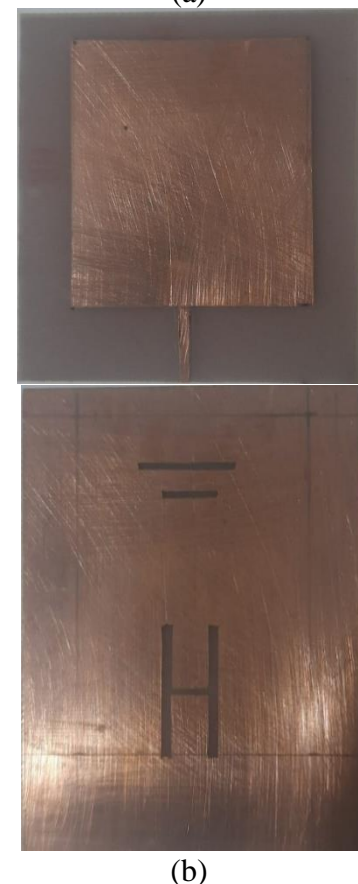
Figure 3 (A) Geometry of Proposed Antenna, (B) Fabricated Antenna - Patch Side, Ground Side
